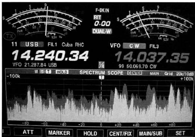
Photo D—A snapshot of the IC-7800 spectrum scope while on 20 meters with the CHA250B. The frequency range displayed is 14.140 to 14.340 MHz. Notice the large number of strong signals across the band.
