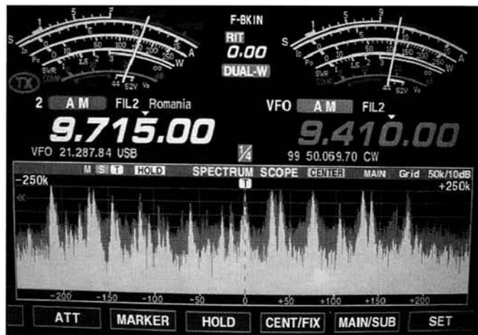
Photo E—A snapshot of the 31-meter shortwave broadcast band. The frequency range displayed is 9.465 to 9.965 MHz. Plenty of strong signals to listen to here!
