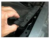
Remove the clips that hold the panel in place to gain access to the fender bolt. Once the bracket is installed and bolted down, replace the clips that hold the panel in place.
