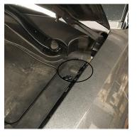
The fender bolt is located under the panel at the front left corner of the engine compartment.
