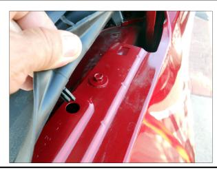
Please Read: Always check for continuity between the bracket and chassis ground. Place the provided star washer between the bracket and fender for grounding and proper alignment.
