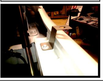
Please Read: Always check for continuity between the bracket and chassis ground. If there is a problem with grounding, place the provided star washer between the bracket and the fender.
