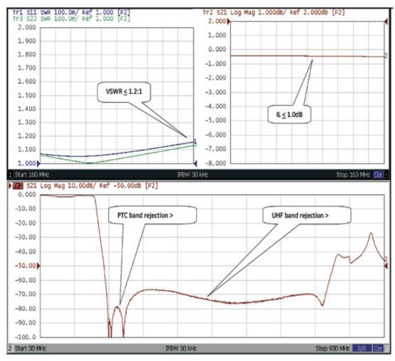
Rejects Unwated RF Signals from: PTC/UHF Bands Filter is designed specfically for locomotive applications
