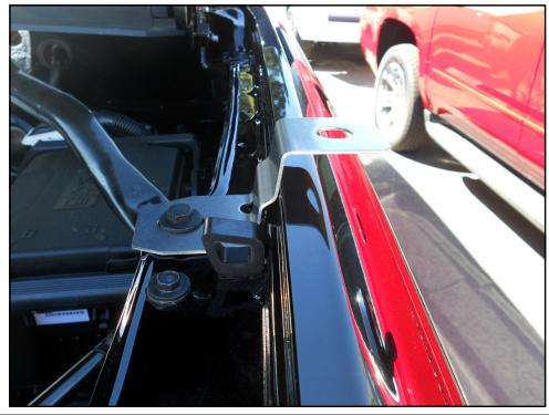
Please Read: Always check for continuity between the bracket and chassis ground. If there is a problem with grounding, place the provided star washer between the bracket and the fender.
