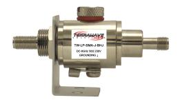
Ventev's TerraWave lightning arrestor is a bi-directional gas discharge tube suppressor that features wide-band operation up to 6 GHz and is rated at IP67. Simply attach the lightning protector to an access point to help protect an entire network, outdoor antennas and other wireless equipment from the build-up of static electricity. It is recommended to use 18 American Wire Gauge (AWG) ground wire.
